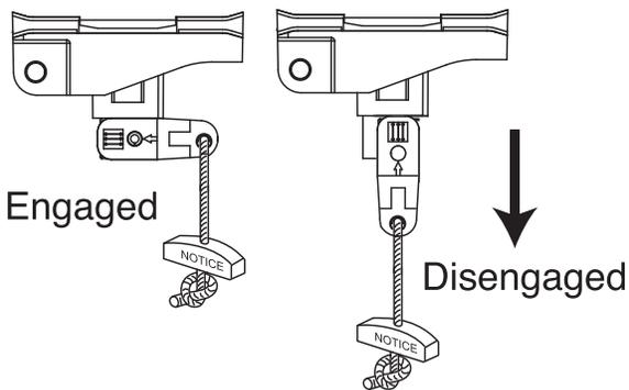
**DO NOT DISENGAGE THE OPENER TO MANUAL OPERATION WITH CHILDREN, PERSONS OR OTHER OBJECTS INCLUDING MOTOR VEHICLES WITHIN THE DOORWAY: (The door is under significant tension and if the door has developed a fault or incorrect tension, it may be unsafe and may fall rapidly.)**
