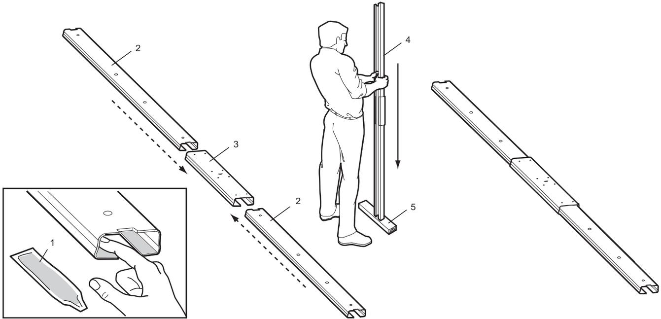
Grease inside edges of rail sections using grease (1). Place rail pieces (2) on flat surface for assembly. All four rail sections are interchangeable. Slide rail brace (3) onto rail section. Connect rail by sliding rail brace onto next rail section. Tap rail assembly (4) on piece of wood (5) until rail sections are flush. Repeat with remaining rail sections.
