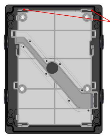
Position the edge of the board which is closest to the fuses under these clips.
