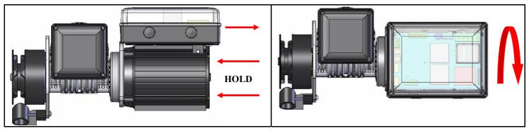
Very carefully rotate both the MCB enclosure and motor to the desired position and replace the two mounting bolts indicated below.
