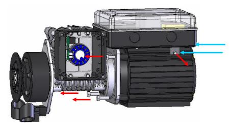
Screws may be located on the side of the MCB enclosure (as shown), or on the end-shield of the motor on later models.
